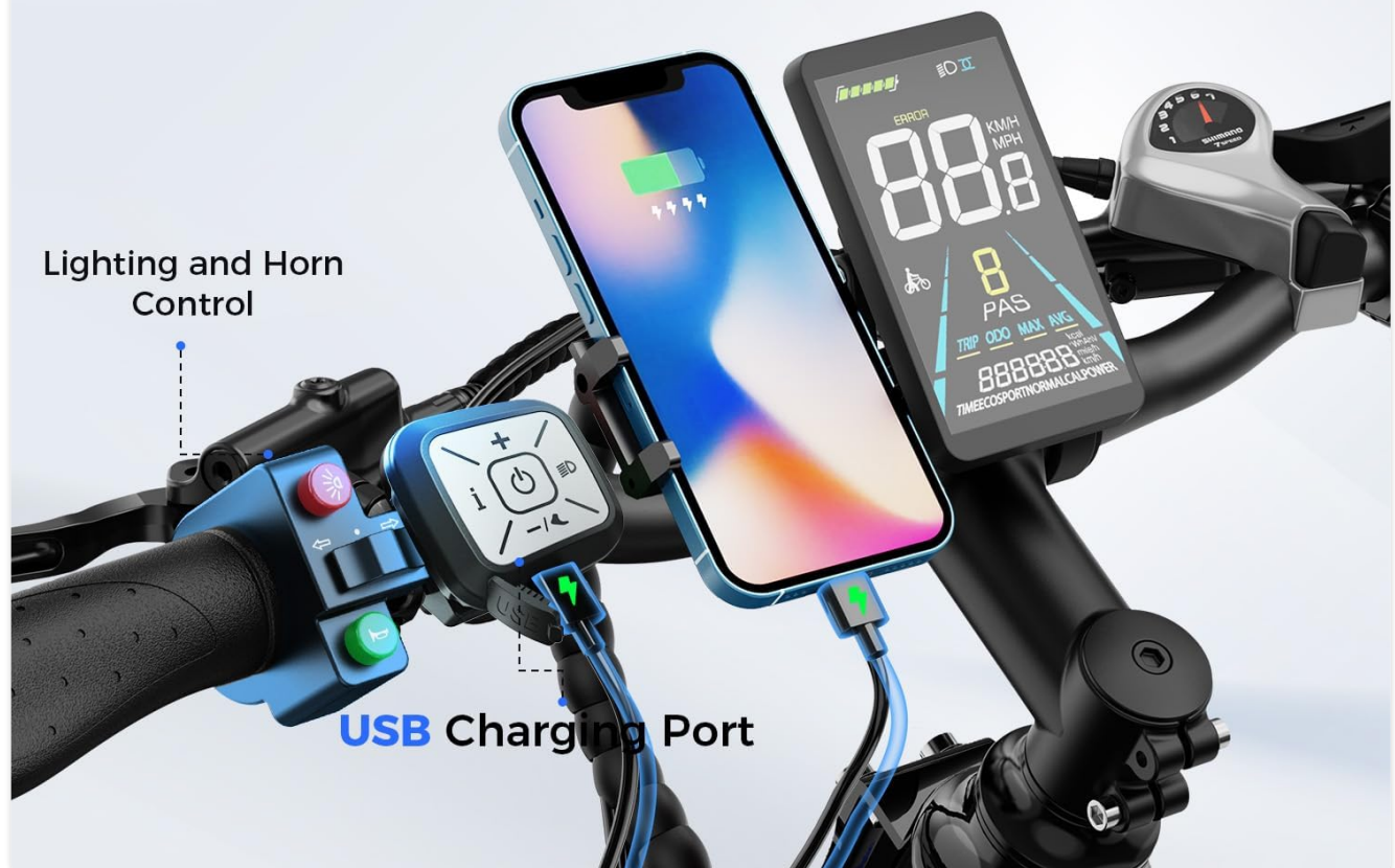
Image 4.1: The Smart M6 LCD display with a USB charging port, showing real-time ride data and integrated controls for lighting and horn.
