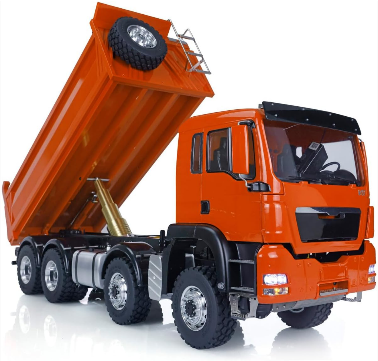
Image 5.2: The dump bed in its fully raised position, powered by the hydraulic system.
