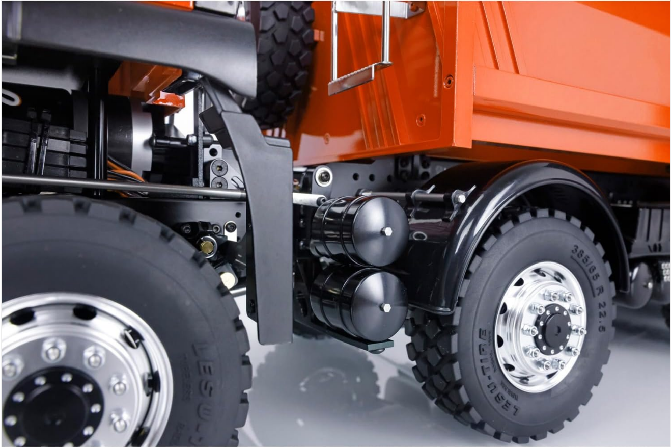
Image 5.1: The all-metal chassis and detailed wheel assembly, designed for durability and traction.
