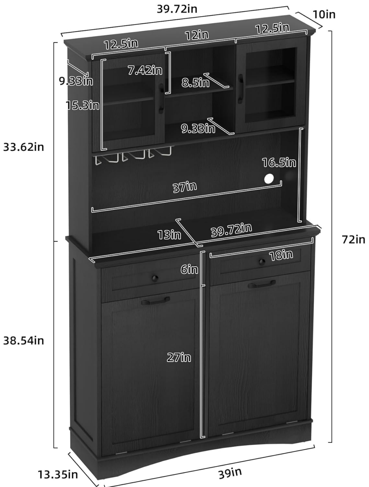
Image: A detailed diagram showing the overall dimensions and internal measurements of the OUTGUAVA Tilt-Out Trash Cabinet, useful for planning placement and understanding component sizes during assembly.
