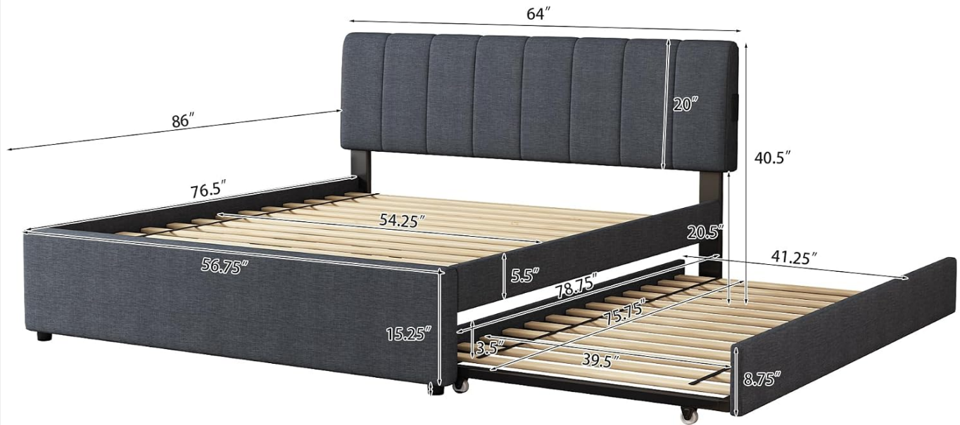
Image 4.1: Dimensional diagram of the Queen Size Upholstered Platform Bed, including the main bed and the pull-out trundle, with key measurements indicated.
