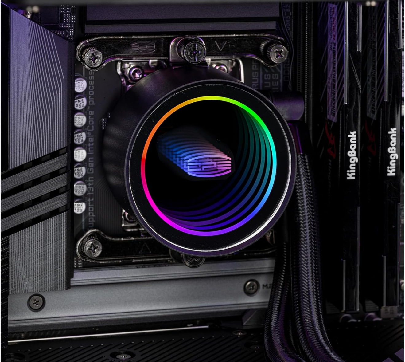
Image: The PCCOOLER DA240 ARGB Liquid CPU Cooler fully installed within a computer system.
