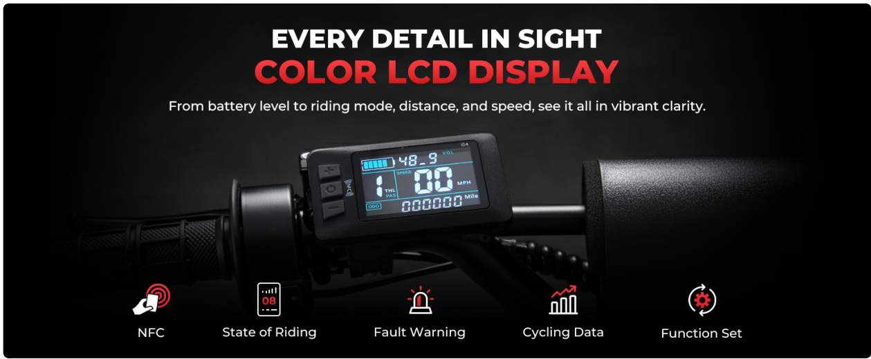
Image 4.3: The color LCD display showing various riding metrics.
