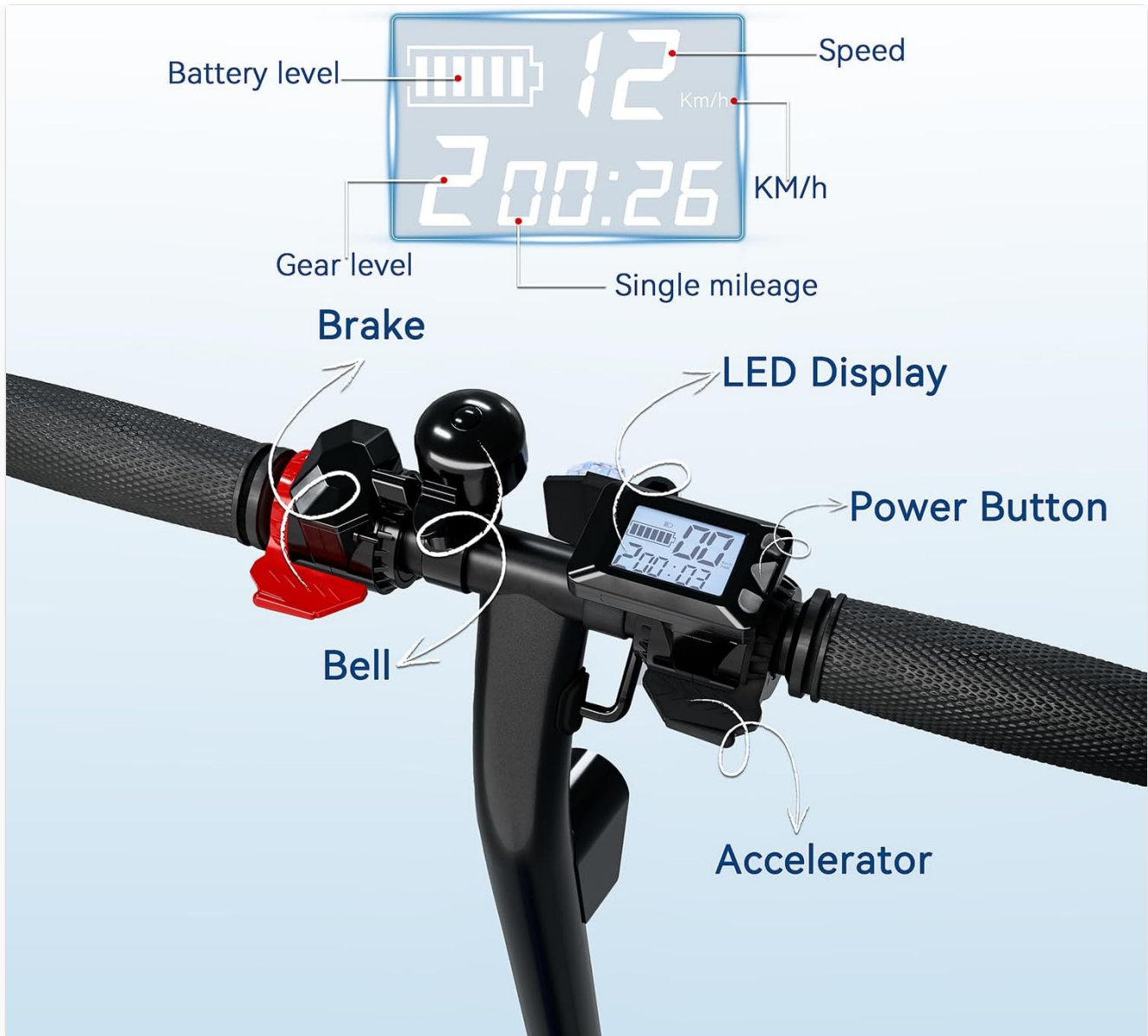
Image: Detailed view of the handlebar controls, including LED display, power button, bell, accelerator, and brake.
