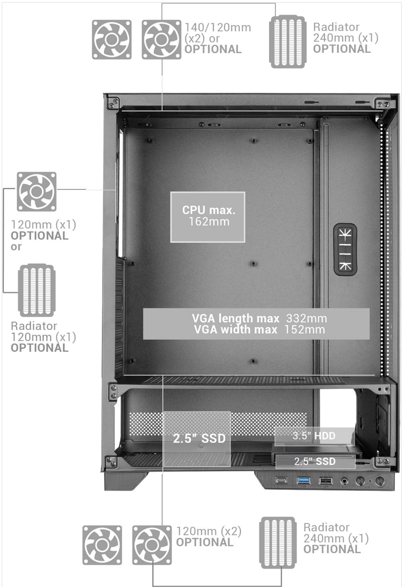
Figure 3: Internal layout showing maximum CPU cooler height (162mm), VGA length (332mm), and VGA width (152mm) clearances, along with fan and radiator mounting points.
