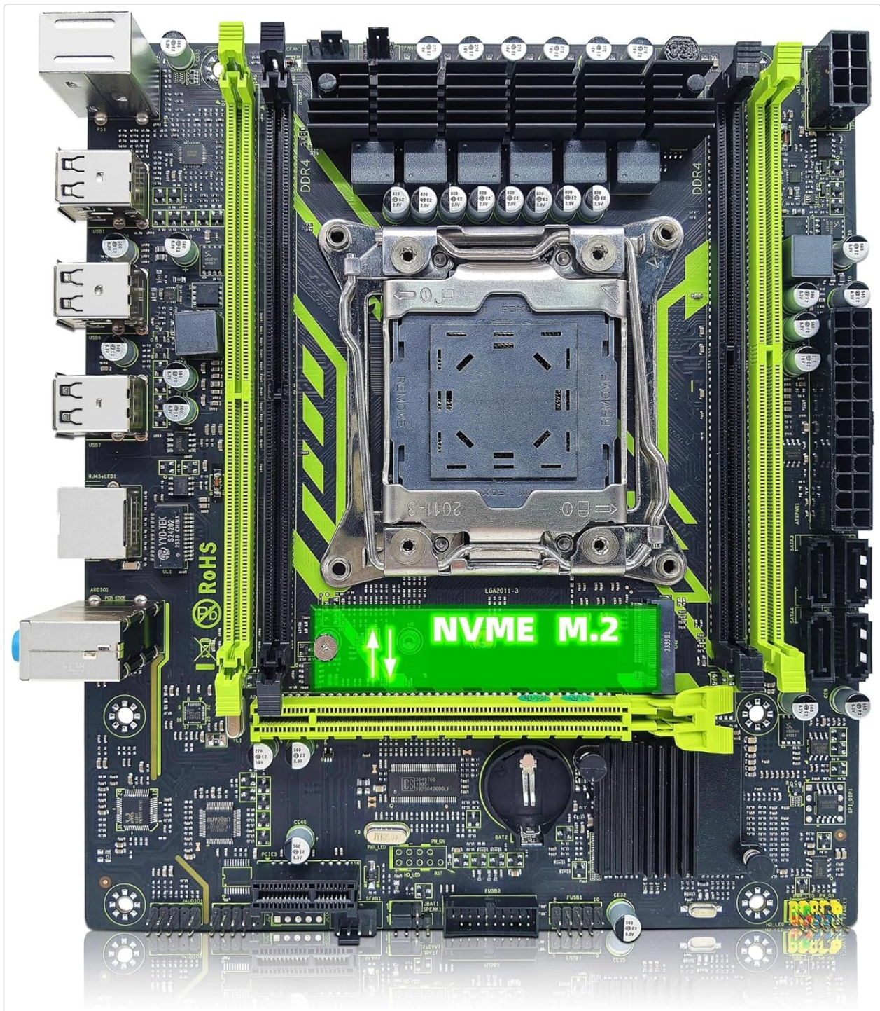
Figure 2.2: ZSUS X99-8D4 Motherboard highlighting the NVMe M.2 slot. This image shows the motherboard with the NVMe M.2 slot clearly visible, indicating its location for SSD installation.
