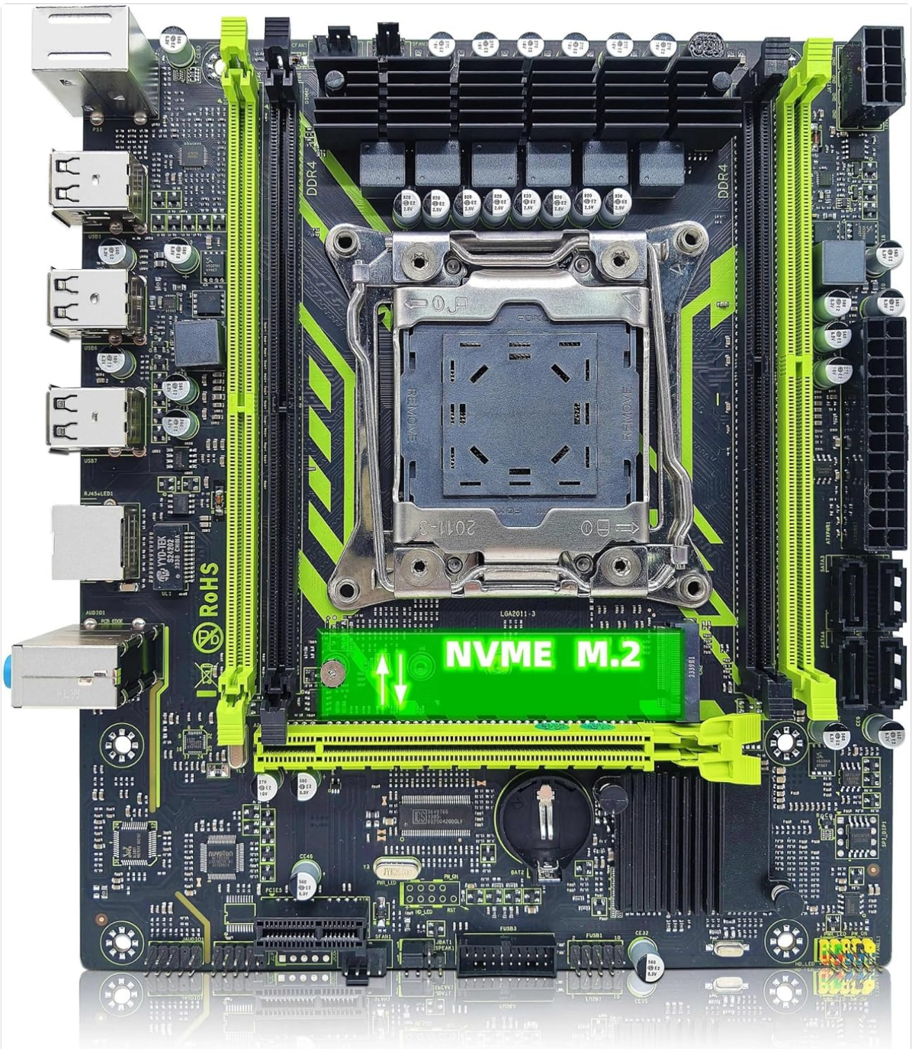
Figure 5.1: NVMe M.2 Slot. This image shows the motherboard with the NVMe M.2 slot prominently highlighted, indicating its location for SSD installation.
