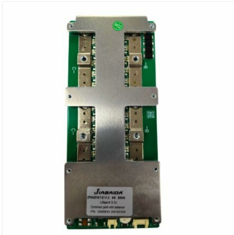
Figure 3: Alternate angled view of the JBD BMS LFP 4S 200A (ZP04S016). This image provides a closer look at the circuit board components and the layout of the power and signal connections.
