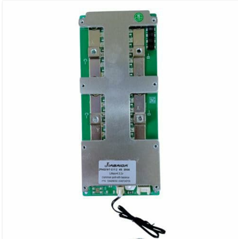
Figure 1: Top view of the JBD BMS LFP 4S 200A (ZP04S016) unit. This image displays the main power terminals, the central heat sink, and the JBD branding label. The balance port connector is visible at the bottom.
