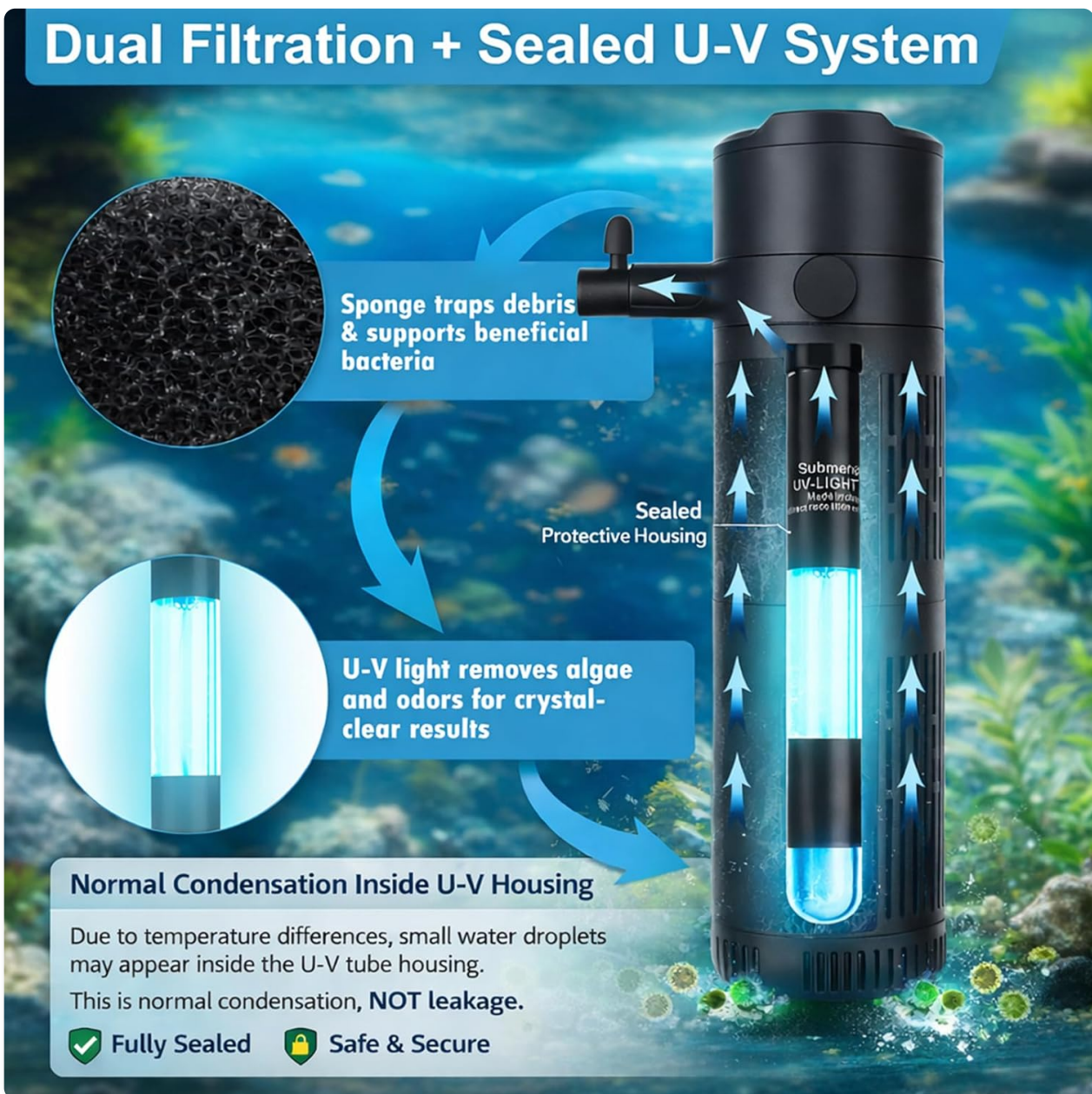
Image: Internal structure showing dual filtration and UV system.
