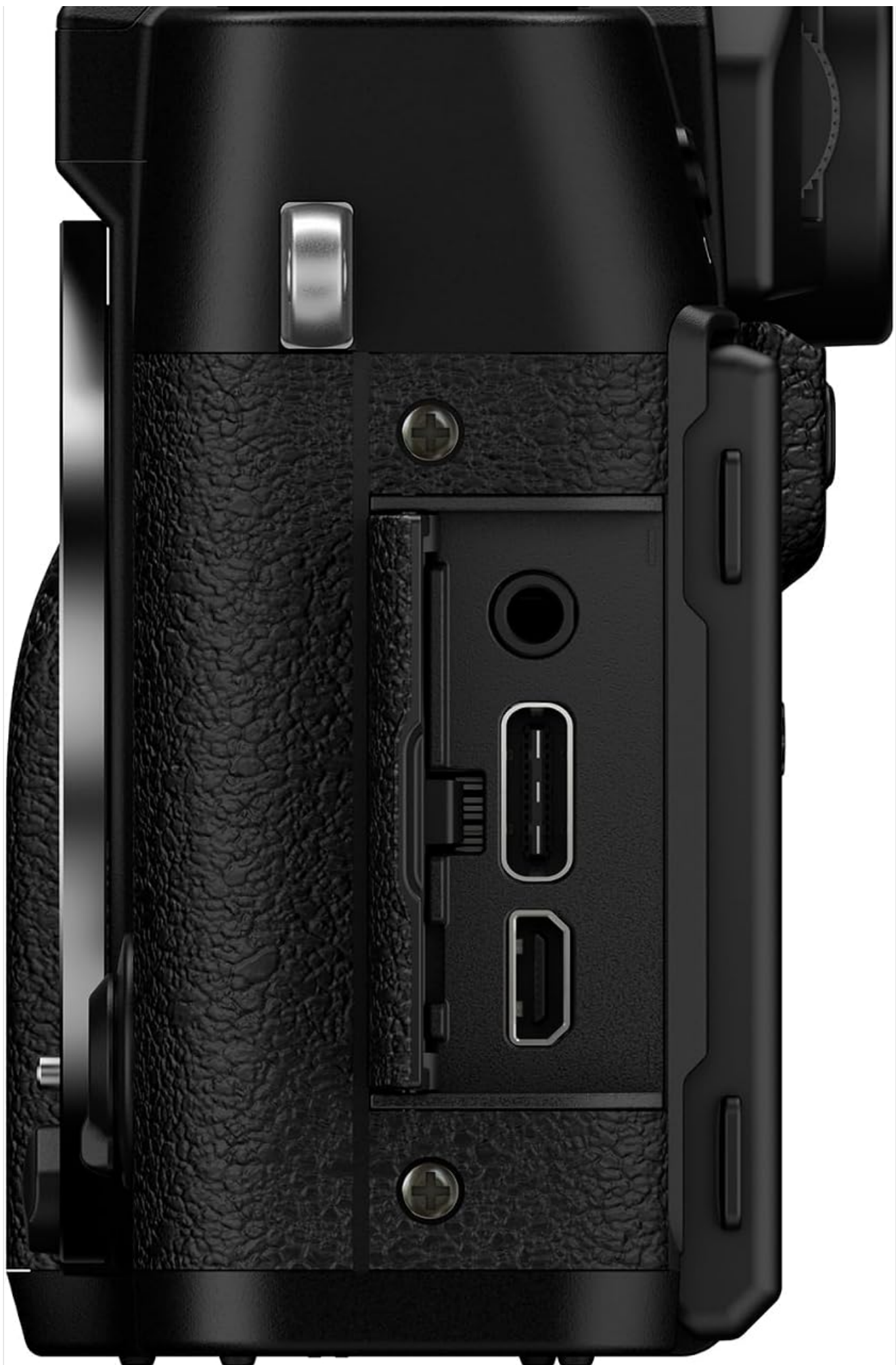
Figure 3.2: Side view of the camera, illustrating the USB Type-C port, microphone input, and other connectivity options.
