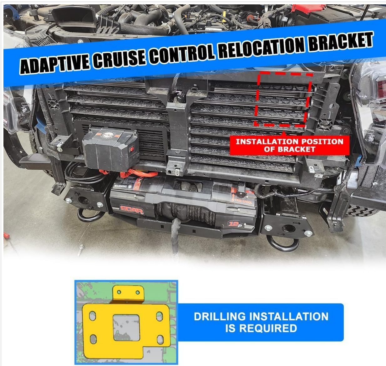
Figure 6: Illustration of the Adaptive Cruise Control relocation bracket and its installation position. The image shows the bracket and notes that drilling is required for its proper mounting.
