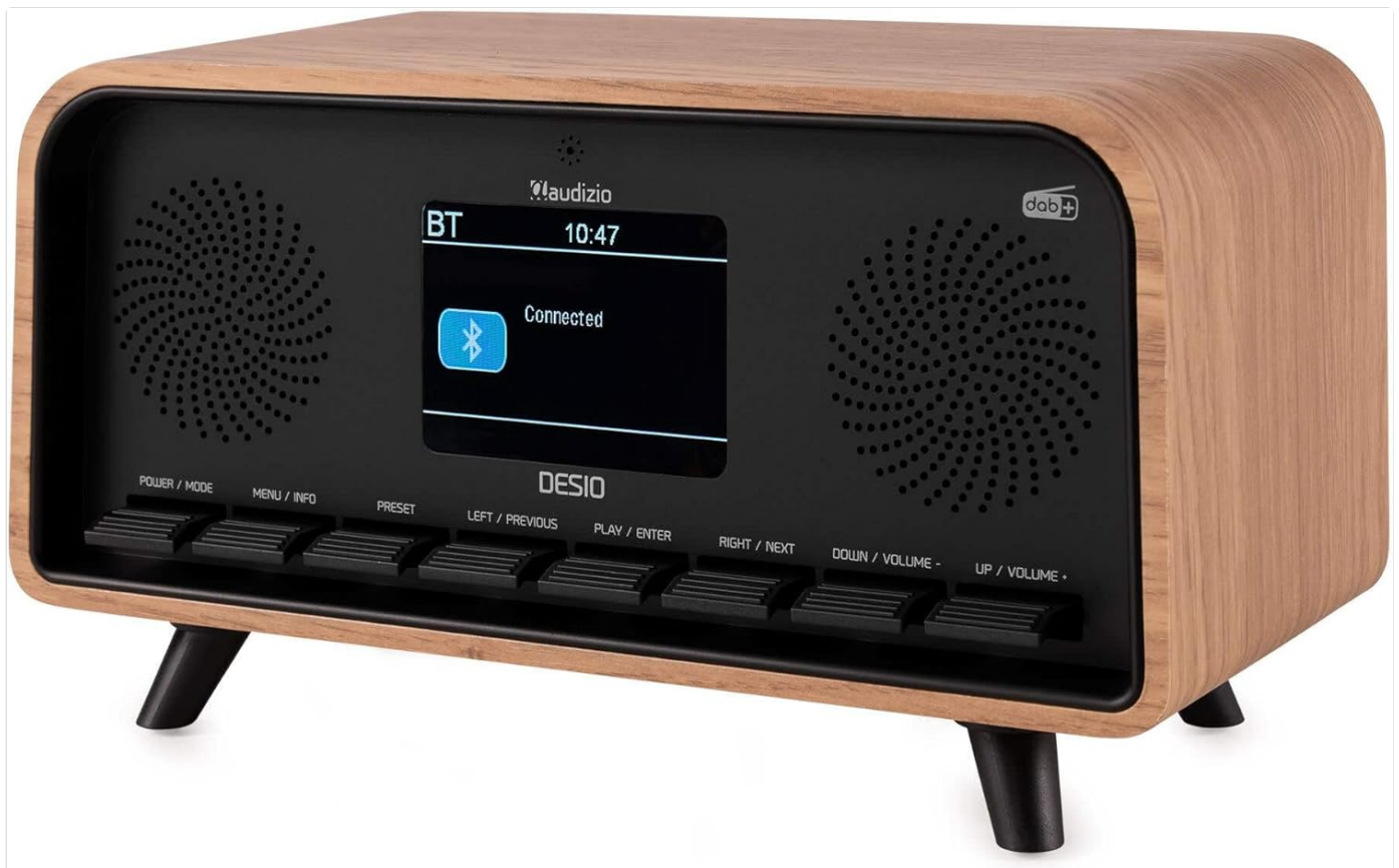
Front view of the Audizio Desio radio, with the display showing 'BT' (Bluetooth) mode and 'Connected' status.
