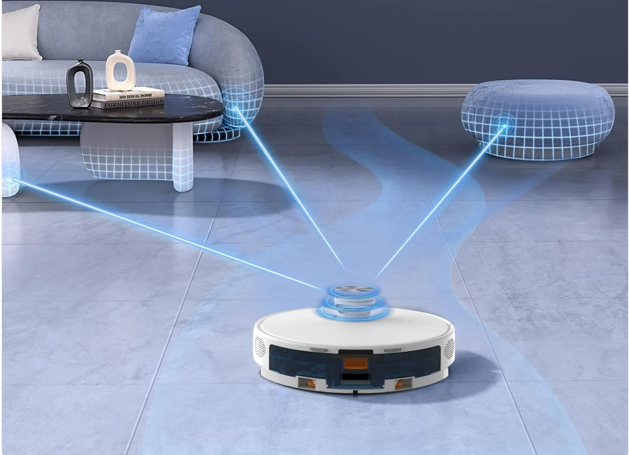
Figure 6: The robot vacuum using LiDAR for precise navigation and mapping.
