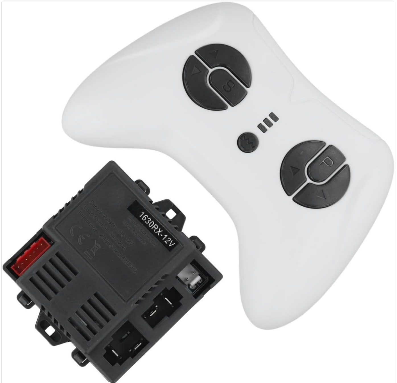
Image: The HanOaki JR1630RX-12V receiver (black box) and its corresponding 2.4G remote control (white). The receiver shows various ports for connection to the vehicle's electrical system.
