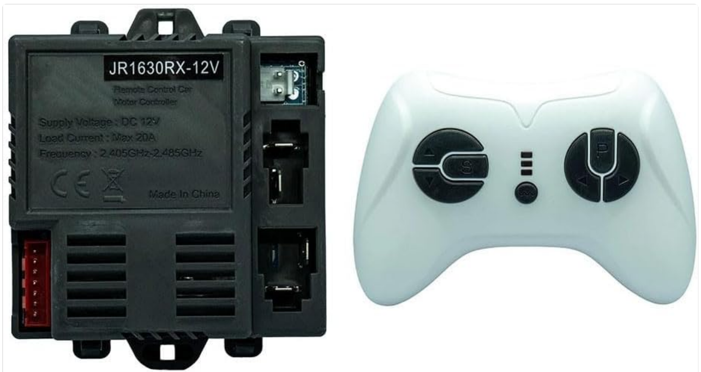
Image: The JR1630RX-12V receiver and 2.4G remote control shown together, illustrating the components involved in the pairing process.
