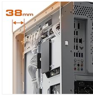
Figure 3.2: Rear interior of the CFV235, illustrating cable management options and locations for 2.5" and 3.5" drive bays.
