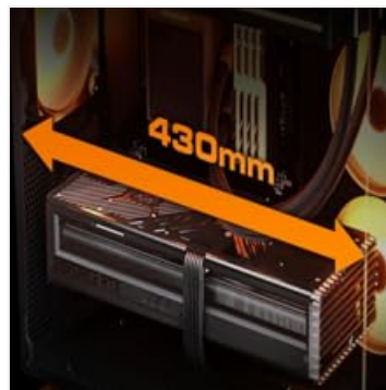
Figure 3.3: Diagram indicating the maximum GPU length of 430mm supported by the CFV235 case.
