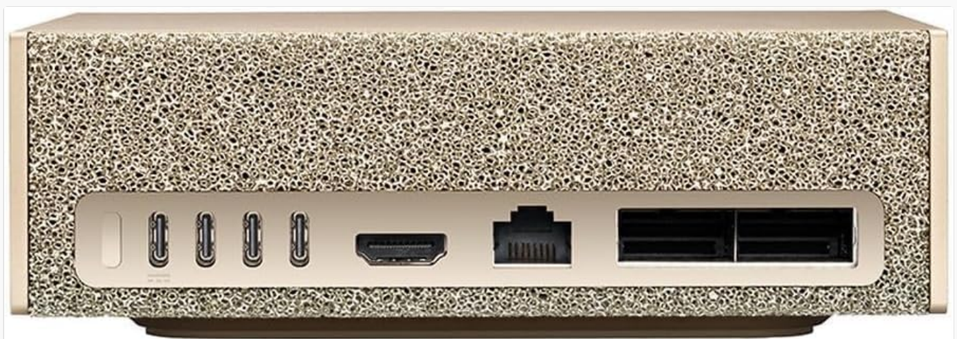
Figure 4.1: Close-up of the textured side panel, indicating ventilation areas.
