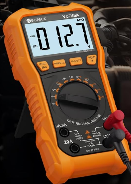
Figure 4.1: Neoteck VC746A Multimeter with highlighted functions. This image illustrates the Neoteck VC746A Digital Multimeter highlighting its comprehensive range of measurement capabilities, including voltage, current, resistance, capacitance, temperature, frequency, duty cycle, non-contact voltage (NCV), live wire detection, diode test, and continuity.
