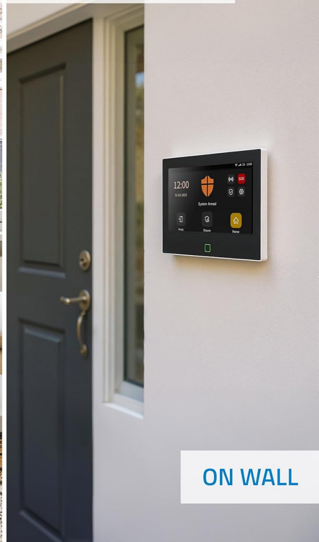
Figure 4: The main control panel interface of the NIVIAN NVS-TOUCHALARM-W, demonstrating options for arming (System Armed), disarming, setting 'Away' mode, and 'Home' mode for tailored security.
