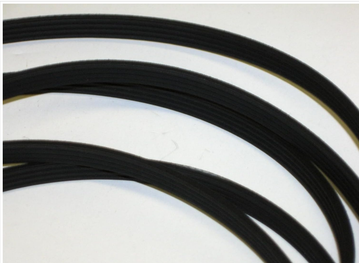
Image: A close-up view of the dryer belt, showing its ribbed surface.
