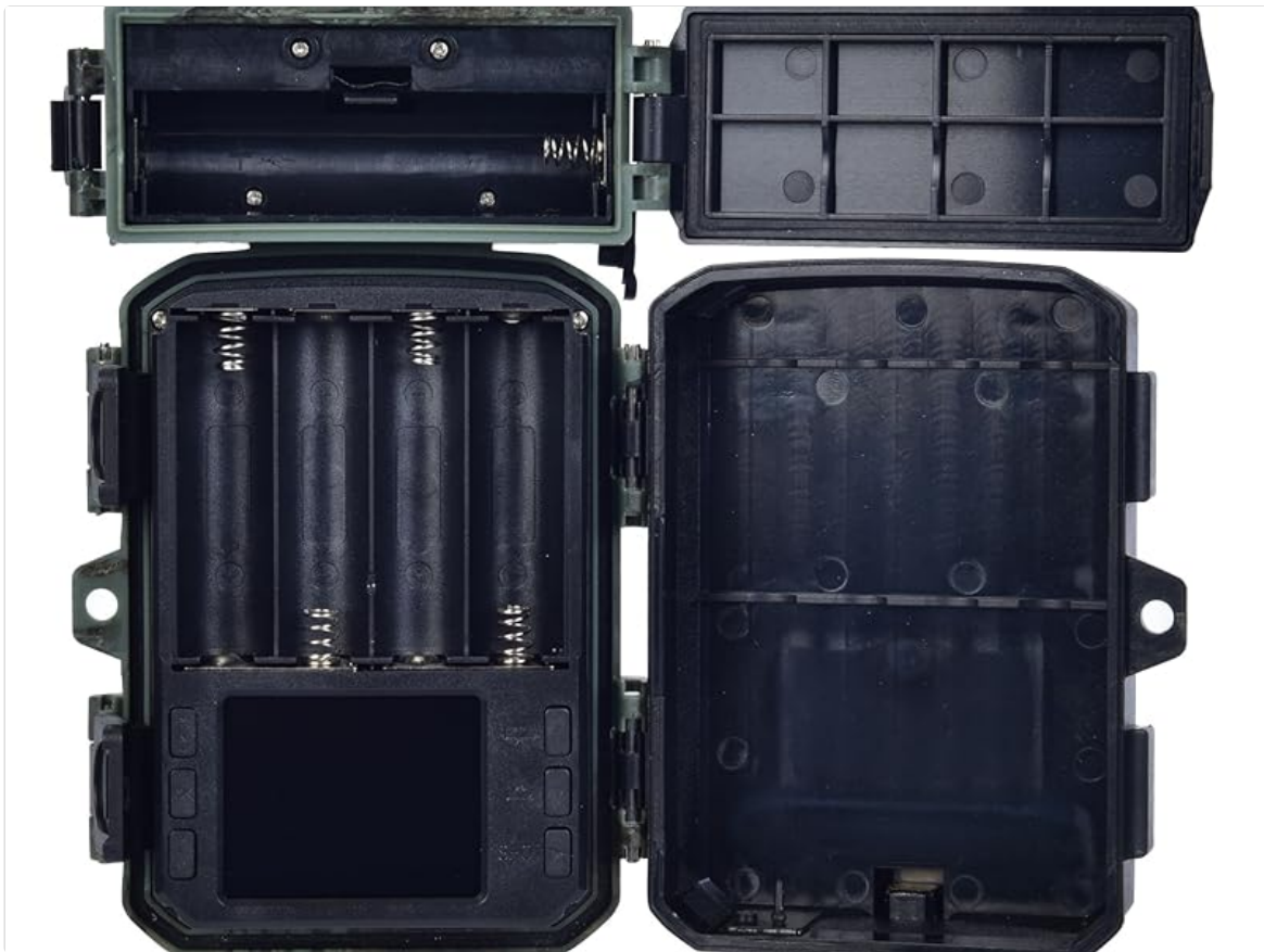
Image: Internal view of the camera showing the battery compartments and SD card slot for proper installation.
