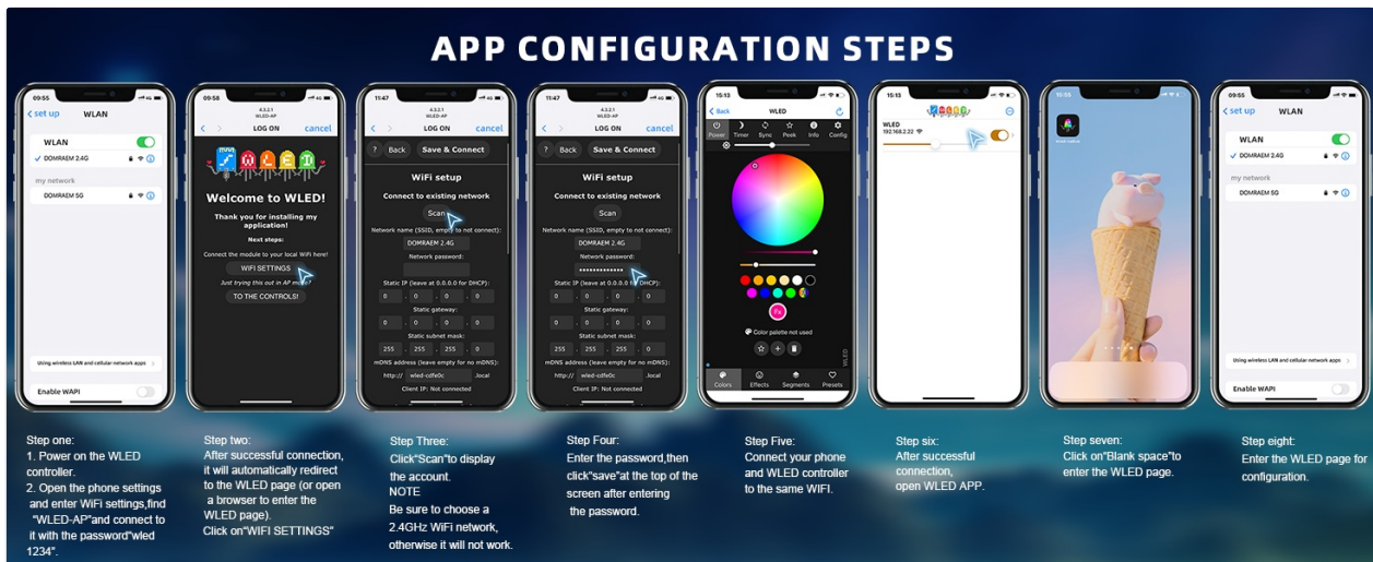
Image: Step-by-step guide for connecting the WLED controller to your home Wi-Fi network via the app interface.
