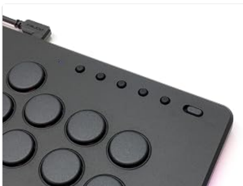
Image 6: The tournament lock switch prevents accidental button presses during gameplay.
