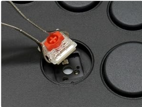
Image 7: Using the key switch puller to remove a hot-swappable switch.
