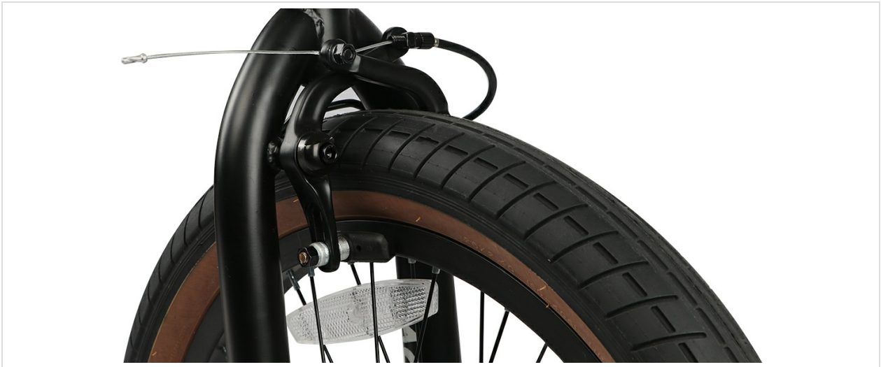
Image: Detailed view of the front U-brake mechanism, highlighting brake pads and cable routing for maintenance checks.
