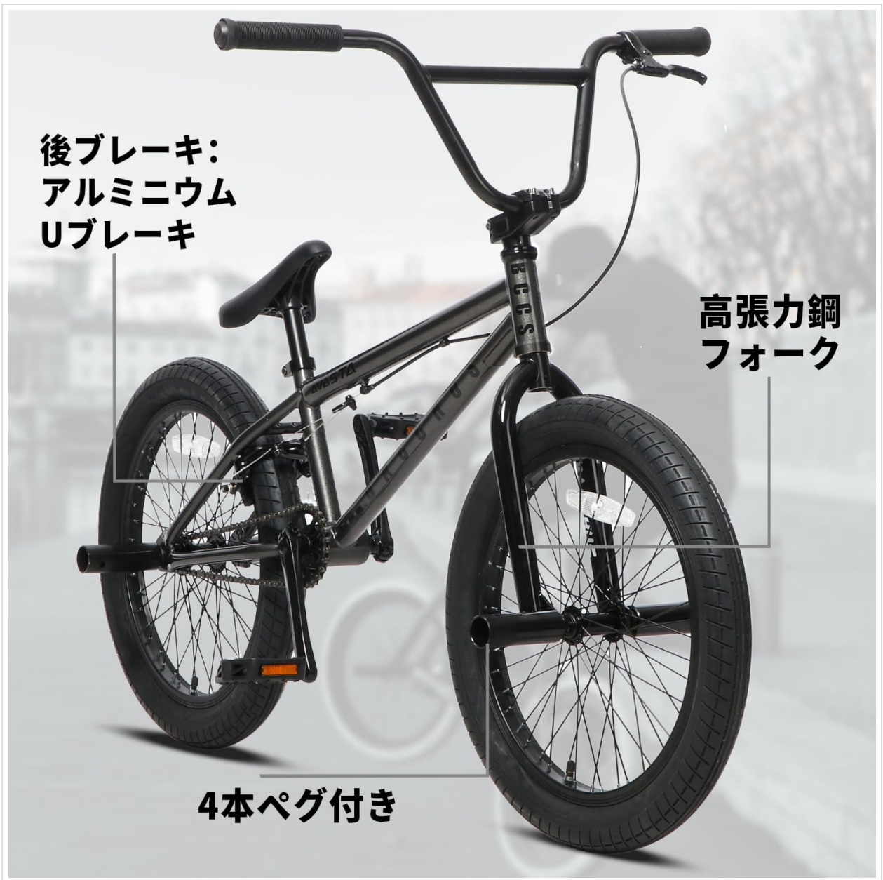
Image: Labeled diagram highlighting key components such as the rear U-brake, high-tensile steel fork, and pegs.
