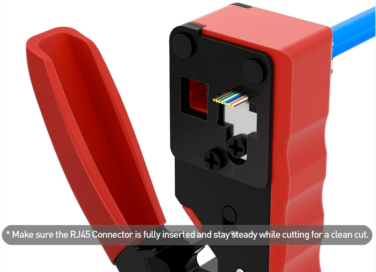
Figure 6: Wires inserted into a pass-through RJ45 connector.
