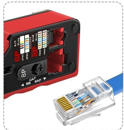
Step 6: Ensure all pins are set and use RJ45 tester to check
