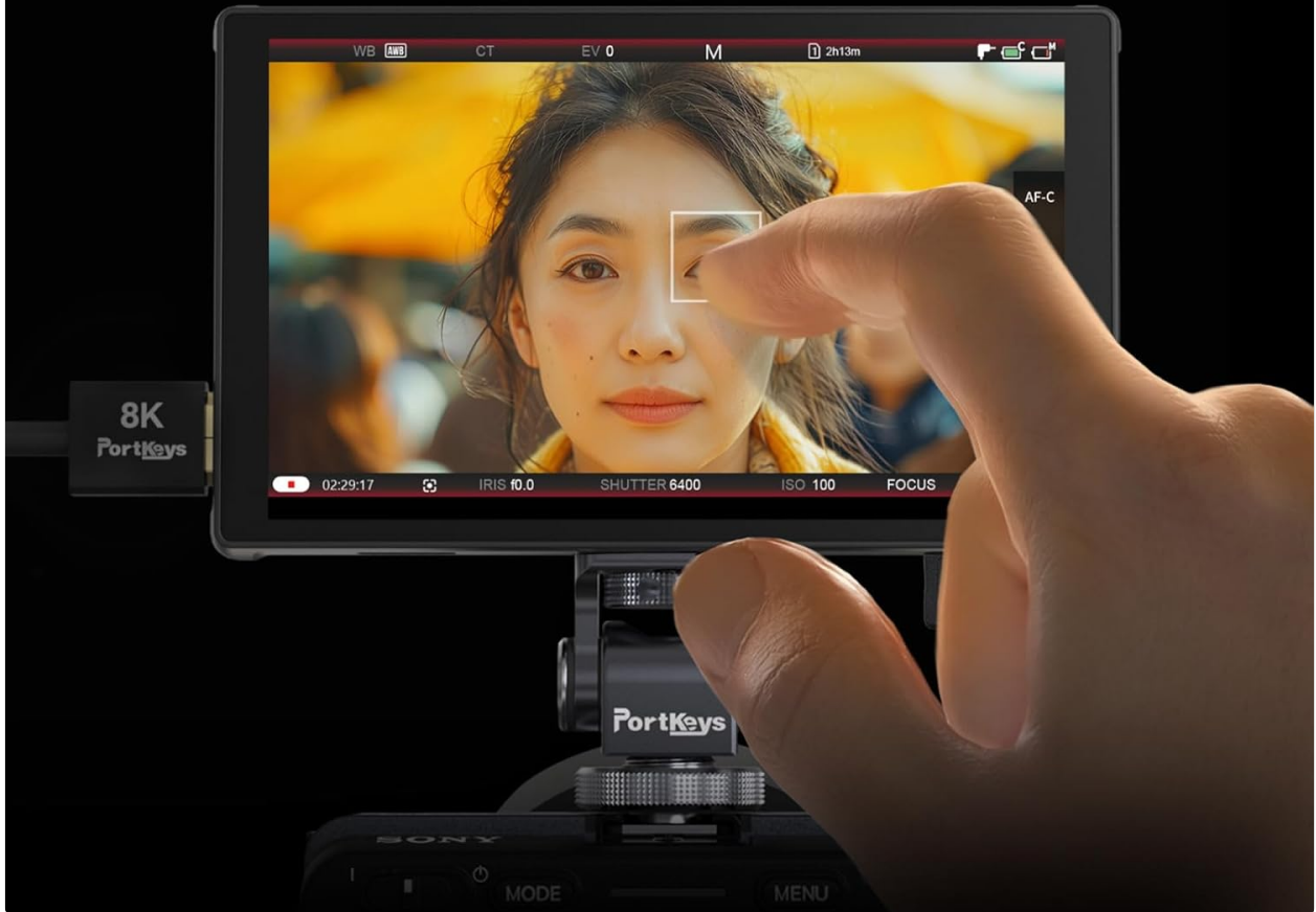
Figure 5.5: Touch Focus Frame in action.
