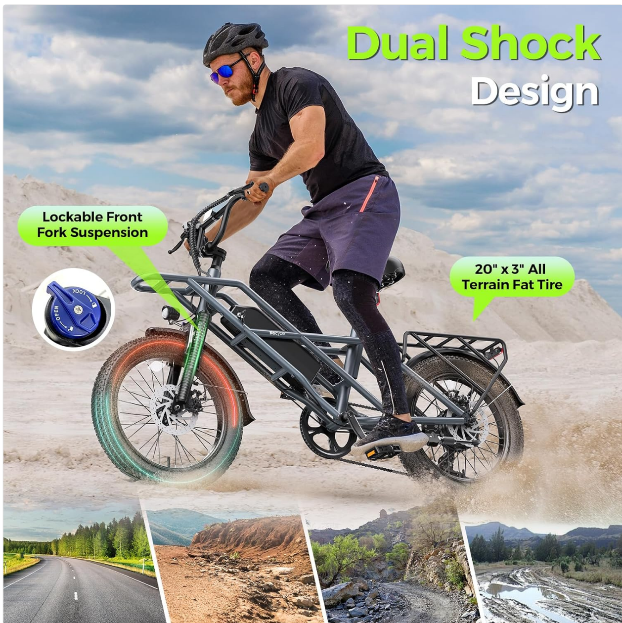
Figure 6: Illustration of the dual shock design with lockable front fork suspension and 20" x 3" all-terrain fat tires, suitable for various road conditions.
