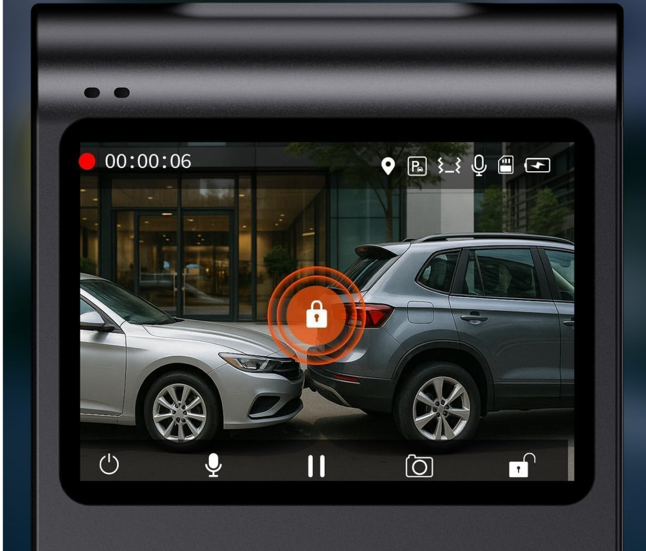
Image 4.3: Automatic collision detection and video lock feature in action.
