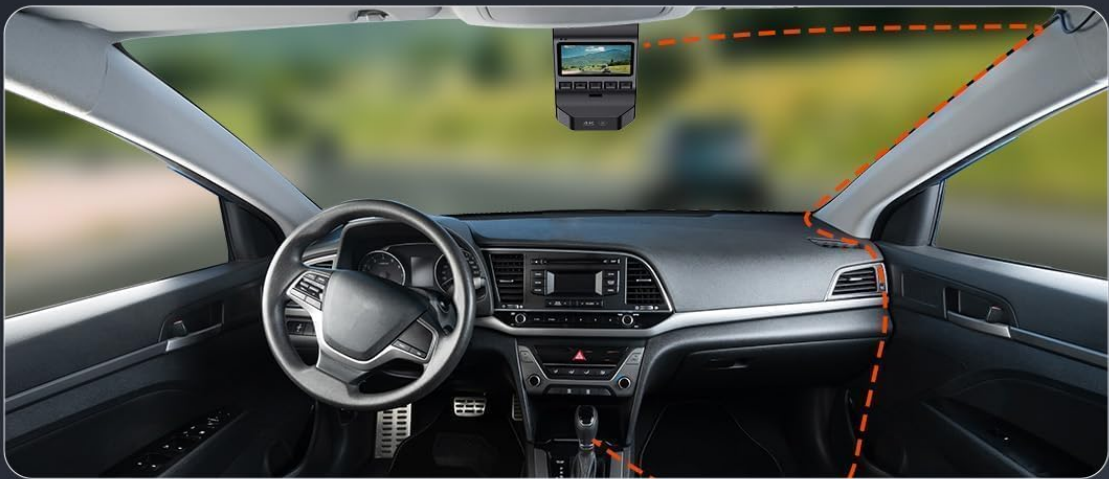
Image 3.1: Visual guide for installing the front and rear dash cameras and routing cables.
