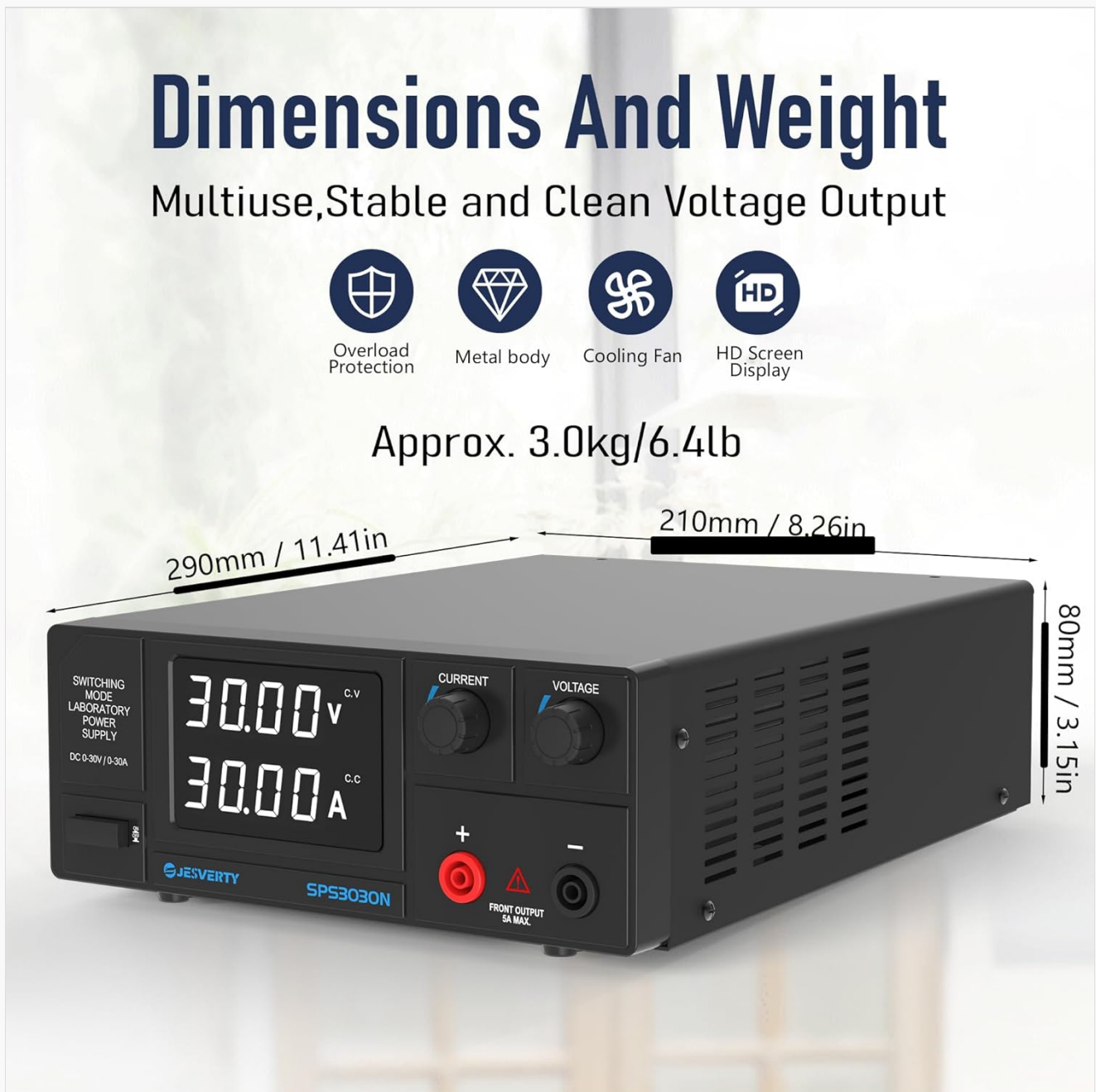
Figure 8.1: Physical dimensions and weight of the Jesvert SPS-3030N DC Power Supply.
