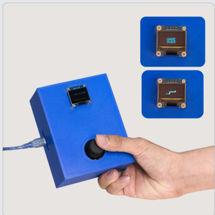
Figure 7: A handheld retro Snake game console, demonstrating an interactive project built with the ESP-32 board and an OLED display.
