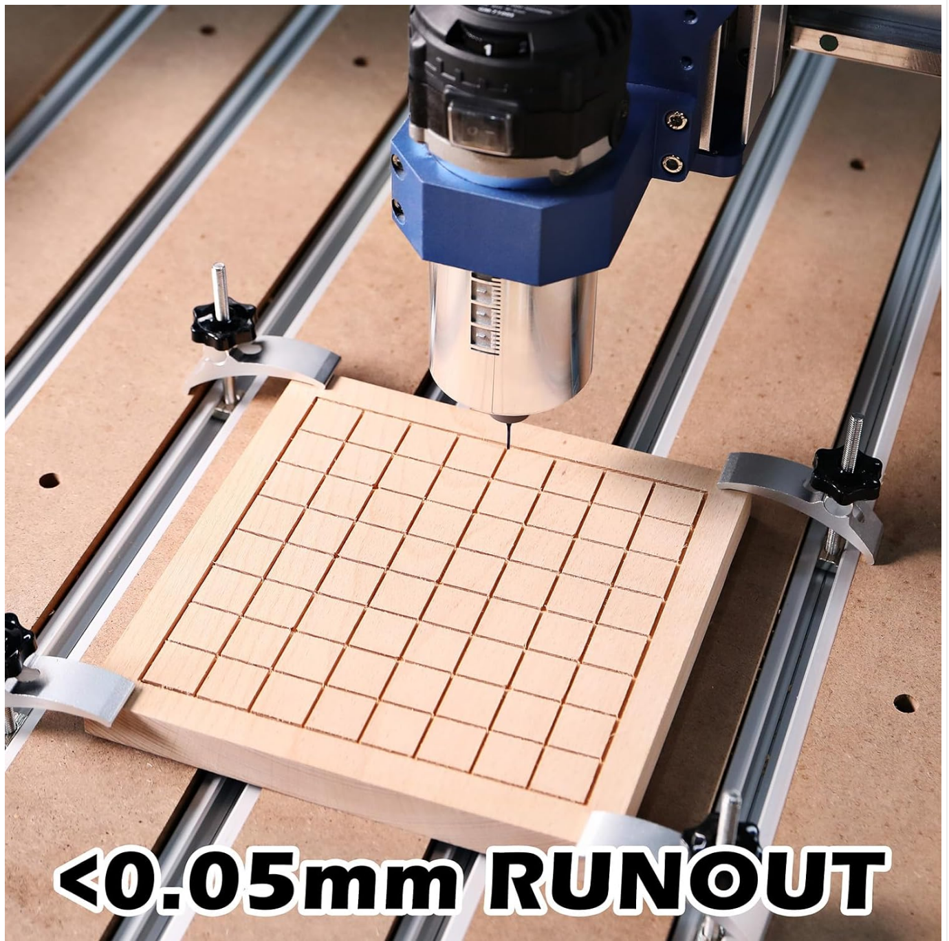
Figure 6: An example of a precise cut with less than 0.05mm runout, highlighting the router's accuracy.
