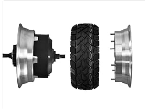
Image 7.1: The split motor design simplifies tire maintenance.
