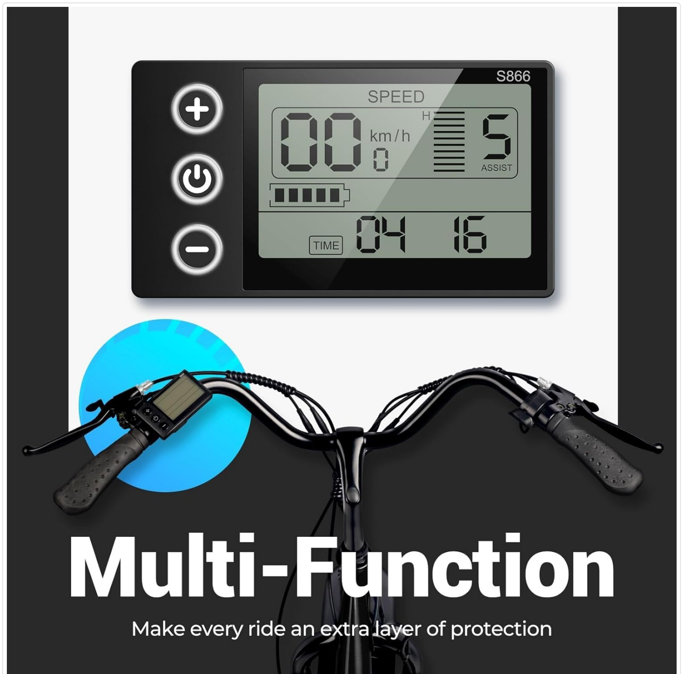
Image: The LCD display showing speed, battery level, distance, and pedal assist level.
