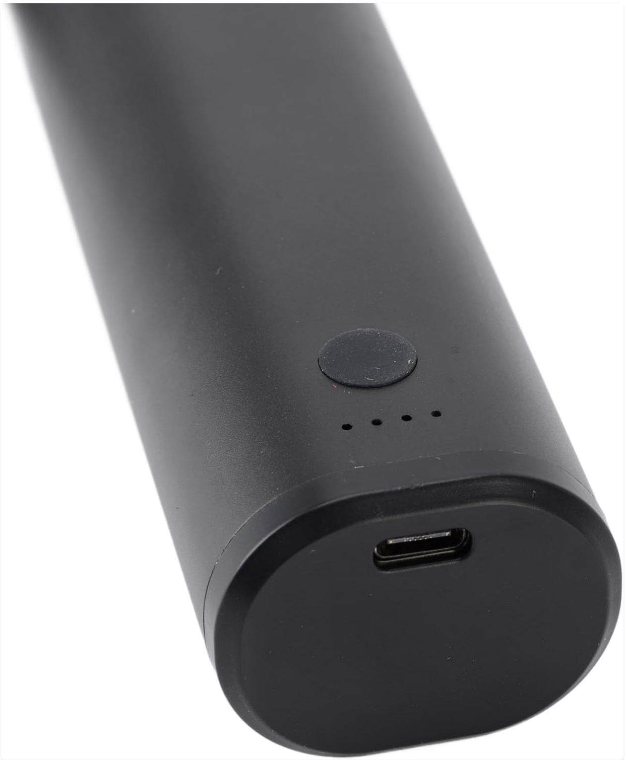
Figure 5.1: USB charging port and battery indicator lights.
