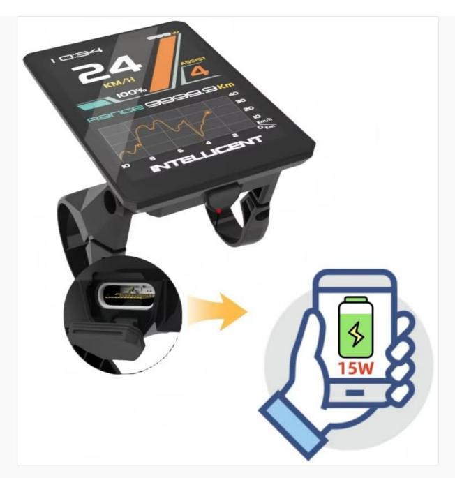
This image highlights the Type-C charging port located on the side of the mGYDY 865C E-Bike LCD Color Display. An arrow indicates its use for charging external devices, such as a smartphone, demonstrating the 15W fast charging capability.
