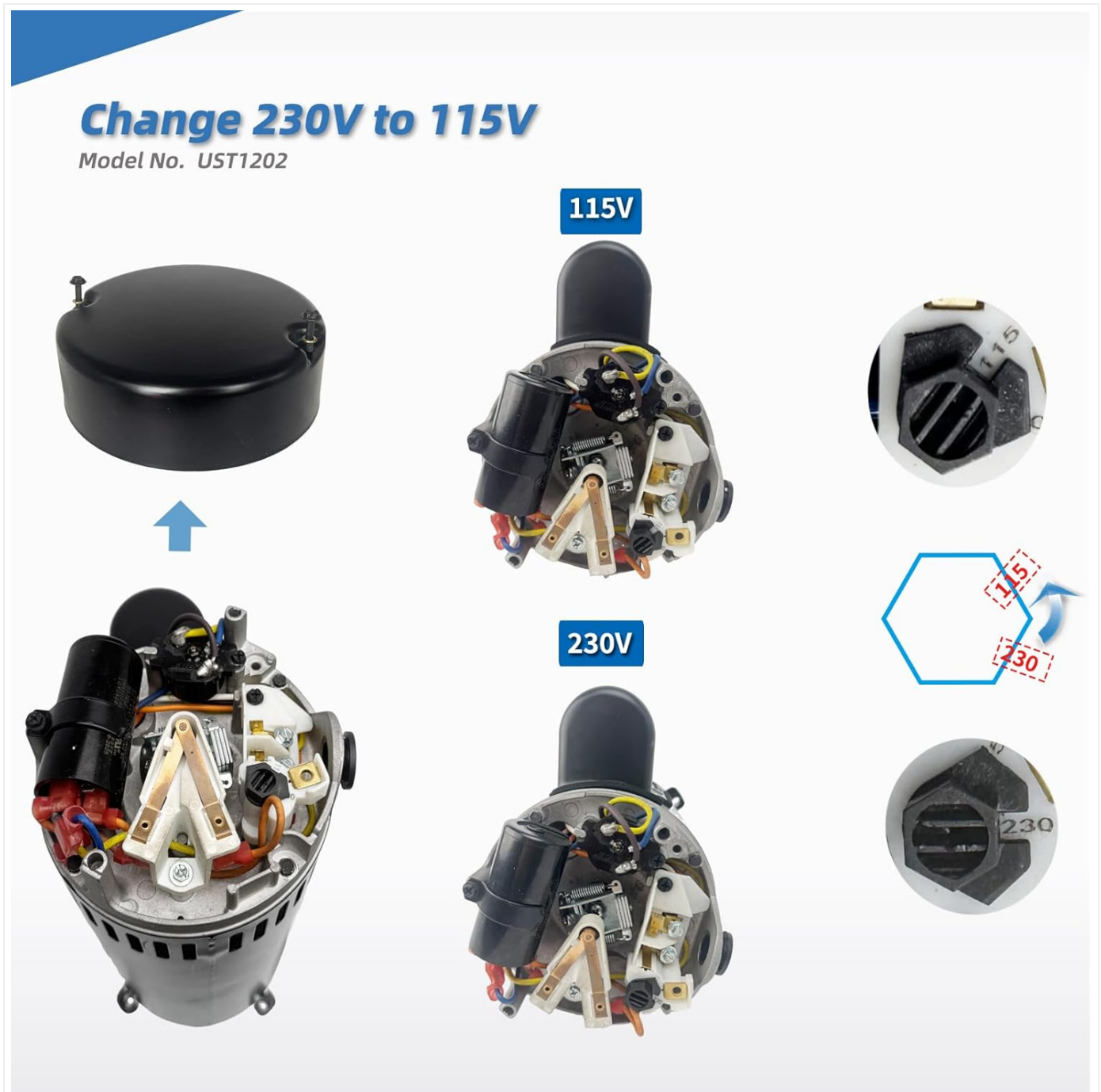
Image 5.1: LEUNGOO UST1202 Voltage Change Diagram. This image illustrates the internal wiring configuration for switching the motor between 115V and 230V operation.
