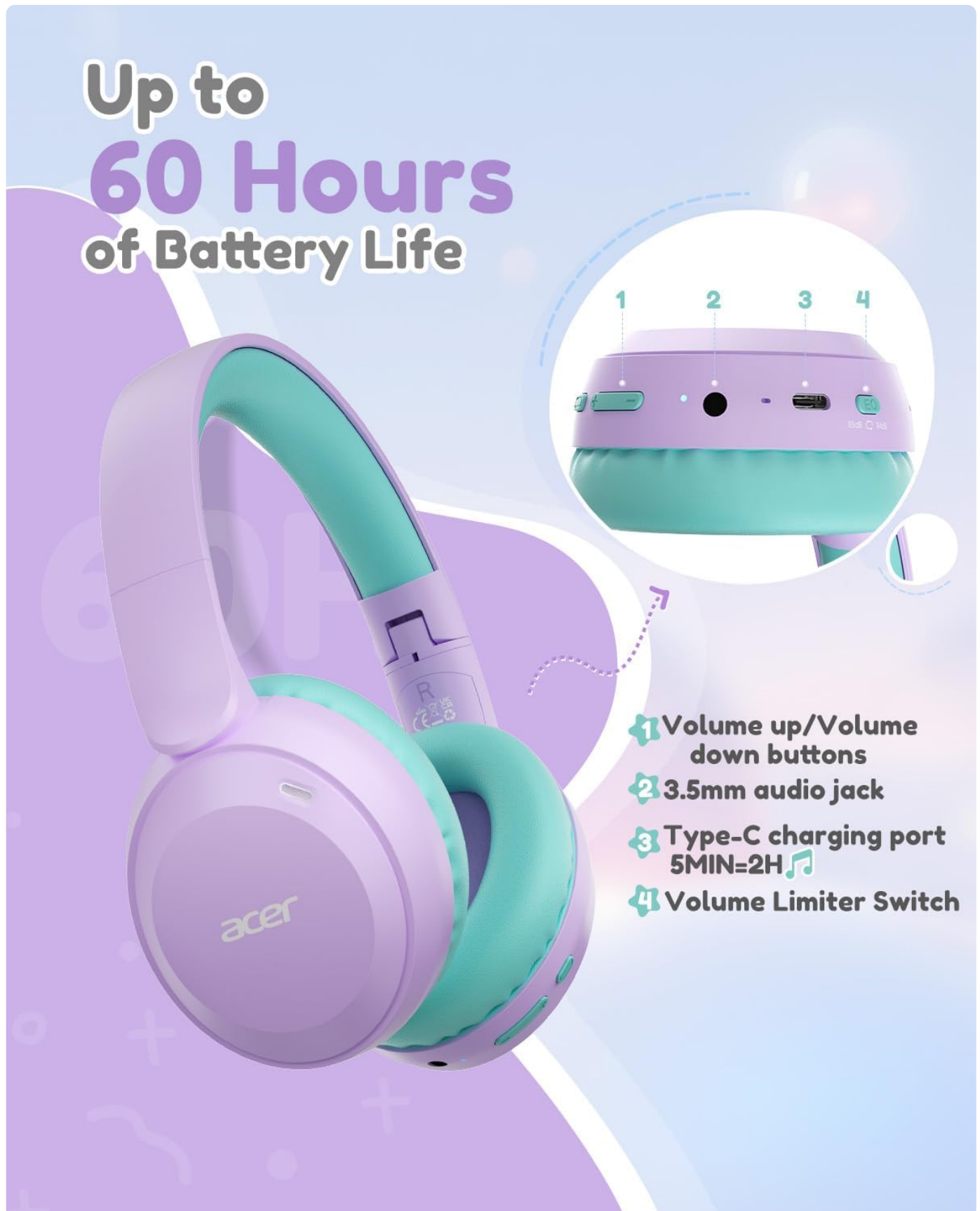
Image: Headphone controls and ports (Volume Up/Down, 3.5mm Jack, Type-C Charging Port, Volume Limiter Switch).
