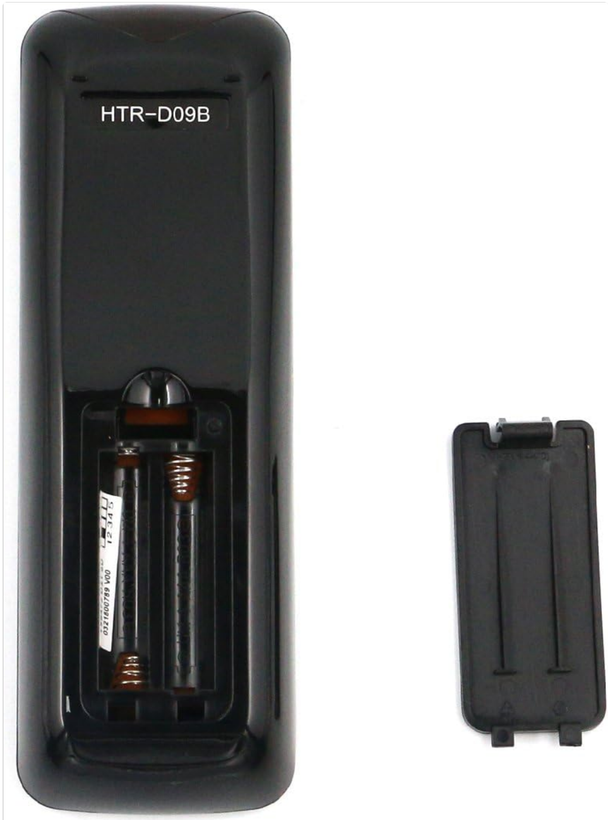
Image: Rear view of the HTR-D09B remote control with the battery compartment open, illustrating the correct orientation for battery insertion. The model number HTR-D09B is visible on the remote's back.
