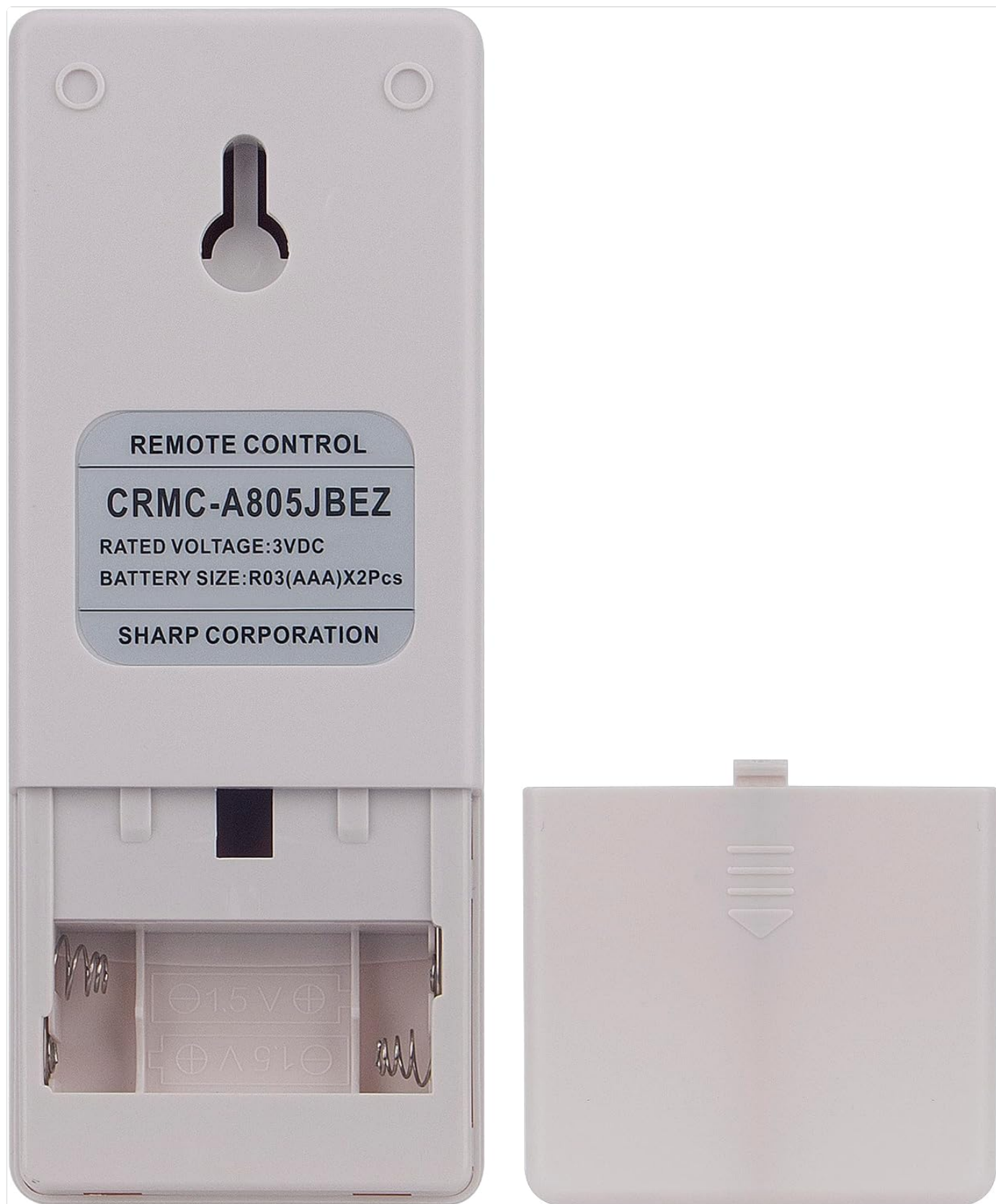
Figure 3: Back view of the remote control with the battery compartment open, showing where to insert AAA batteries.
