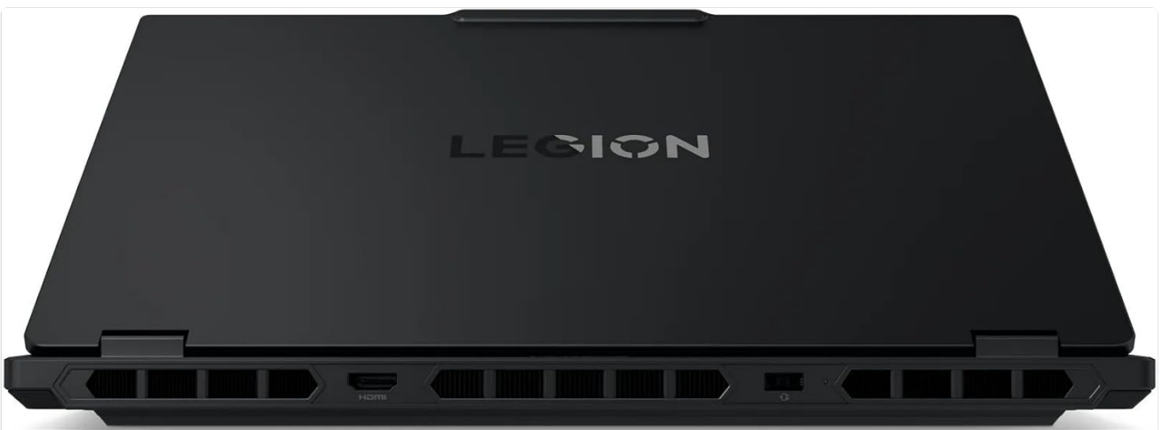
Figure 5: Rear ports including HDMI, RJ-45 (Ethernet), and power input.
