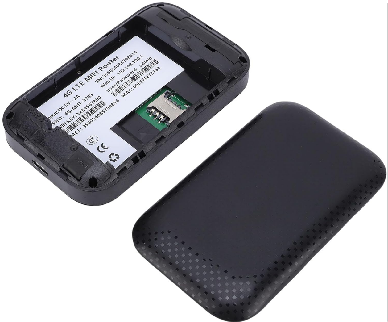
Image: The mobile hotspot with its back cover removed, showing the SIM card slot and internal components.
