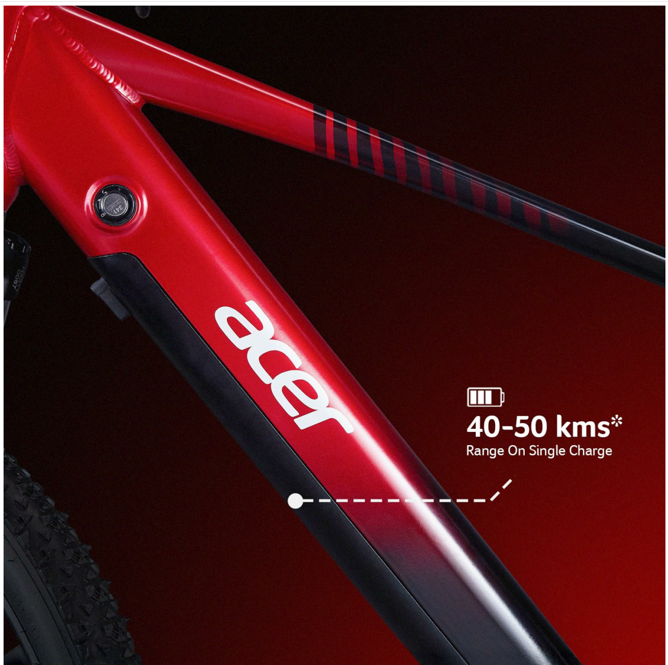
Figure 5.1: Close-up view of the in-frame 9Ah removable lithium battery, which provides a range of 40-50 km on a single charge.
