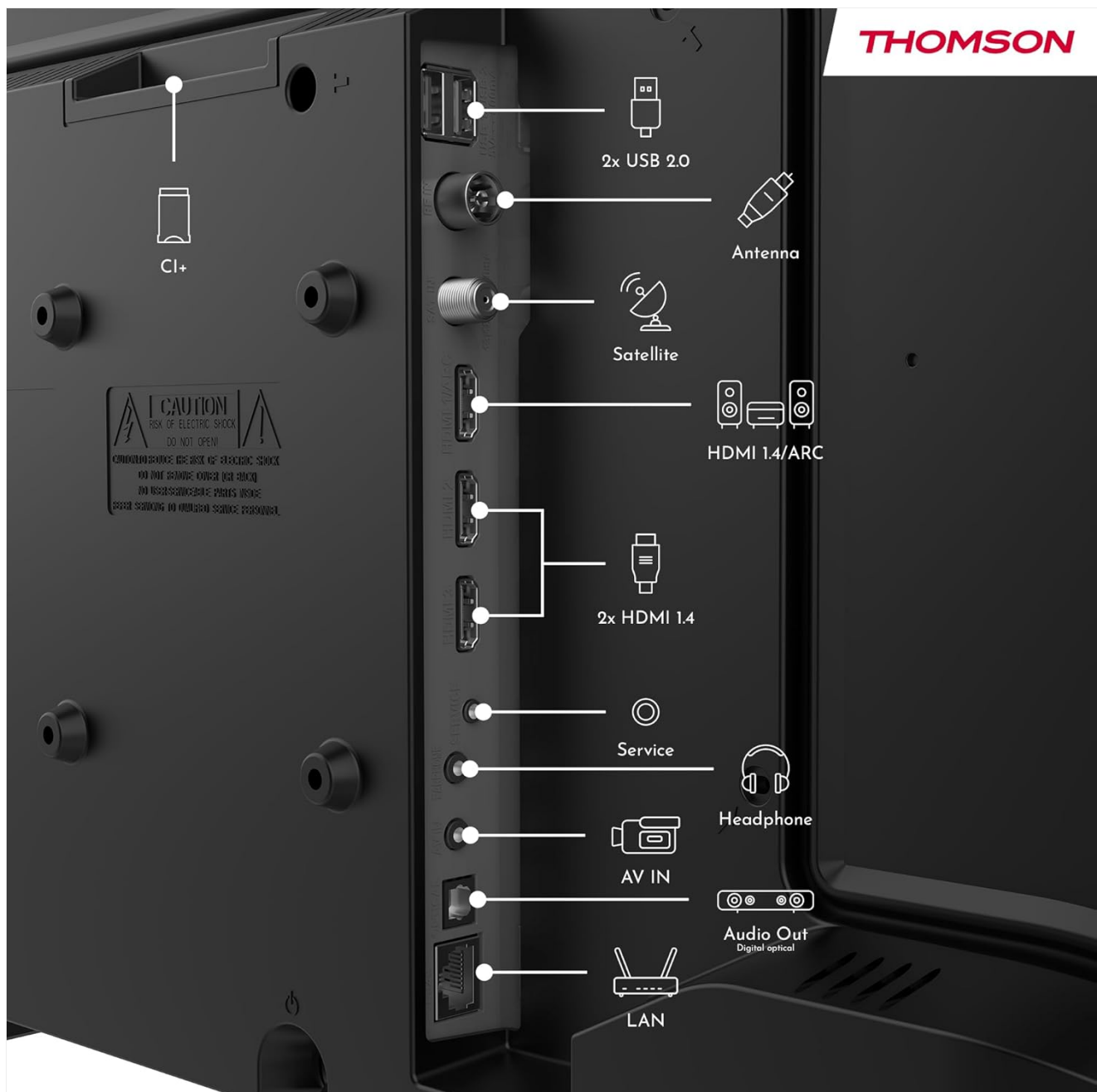
Image 3: Detailed view of the TV's rear connection panel. Ports include CI+, 2x USB 2.0, Antenna input, Satellite input, HDMI 1.4/ARC, 2x HDMI 1.4, Service port, Headphone output, AV IN, Digital Optical Audio Out, and LAN (Ethernet) port.
