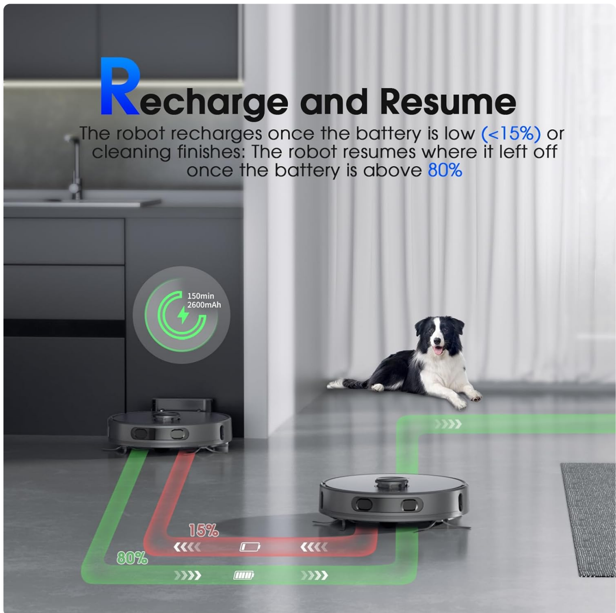
Figure 10: The D60S robot vacuum demonstrating its recharge and resume function, showing the path to the charging station when battery is low (below 15%) and resuming cleaning once charged (above 80%).
