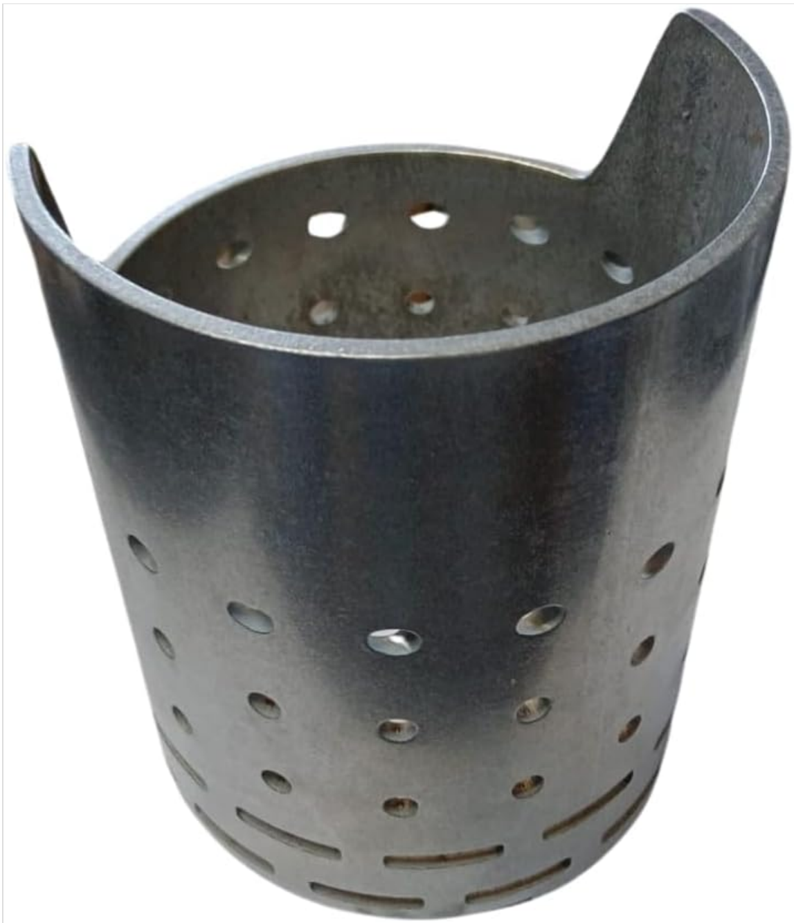
Figure 2: Angled perspective of the crucible. This view provides a better understanding of the internal design and the distribution of the air holes.
