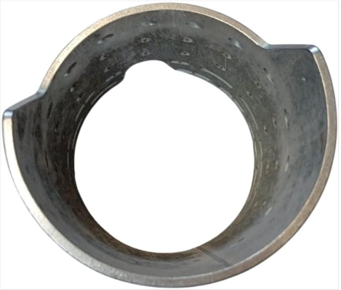
Figure 3: Top view of the crucible. This image illustrates the circular opening where pellets are fed and the shape of the upper rim.
