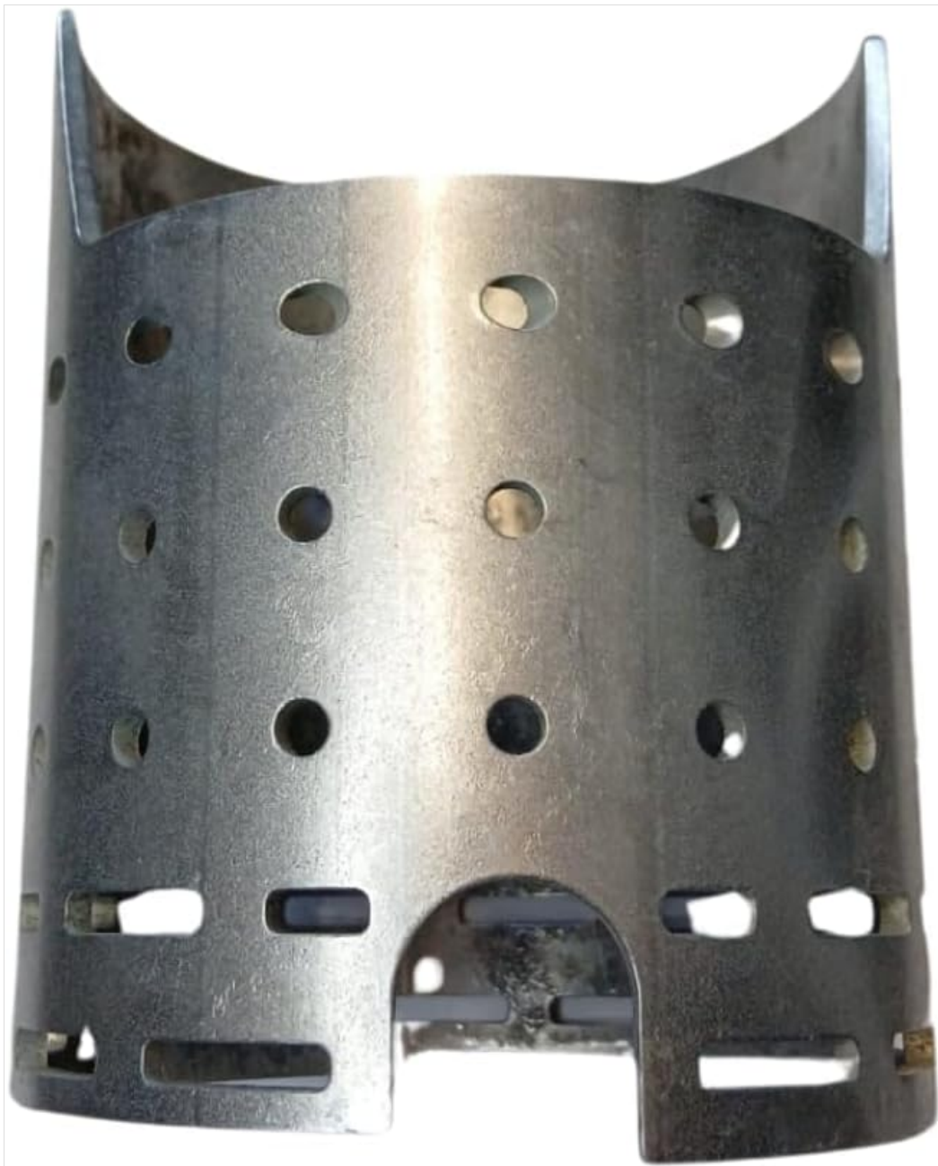
Figure 4: Side view of the crucible. This perspective highlights the full height of the component and the specific design of the air slots at its base.
