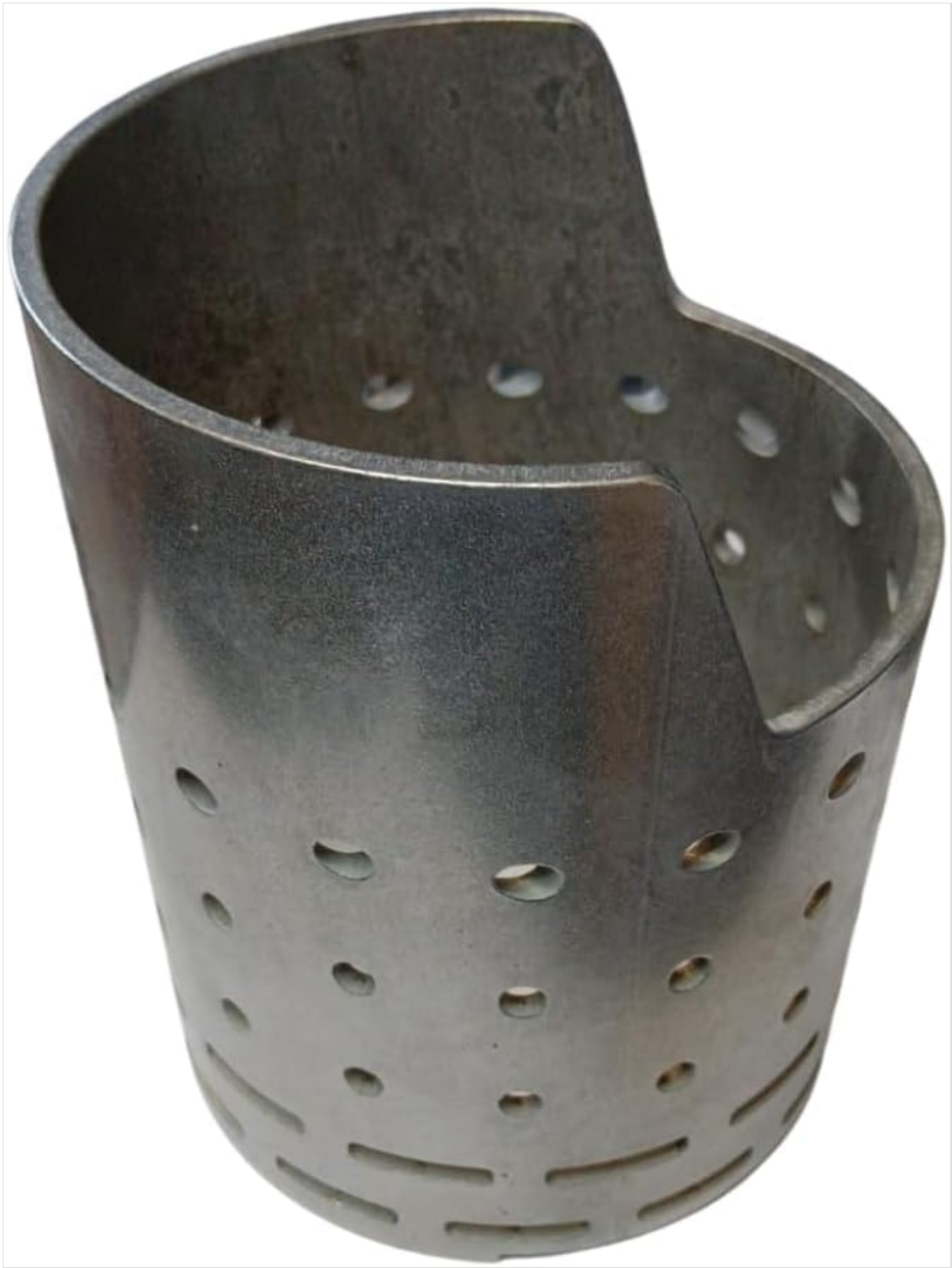
Figure 1: Front view of the steel crucible. This image displays the overall cylindrical structure with perforations for airflow and the distinctive upper opening.
