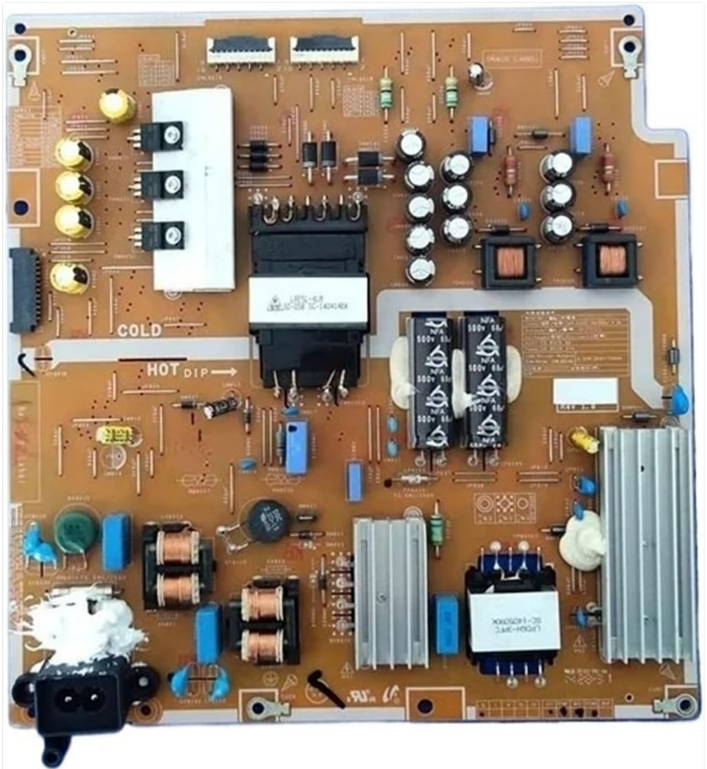
Figure 1: Top view of the RXCWWZQQ BN44-00715A Power Supply Board, showing the overall layout of components and circuitry.
