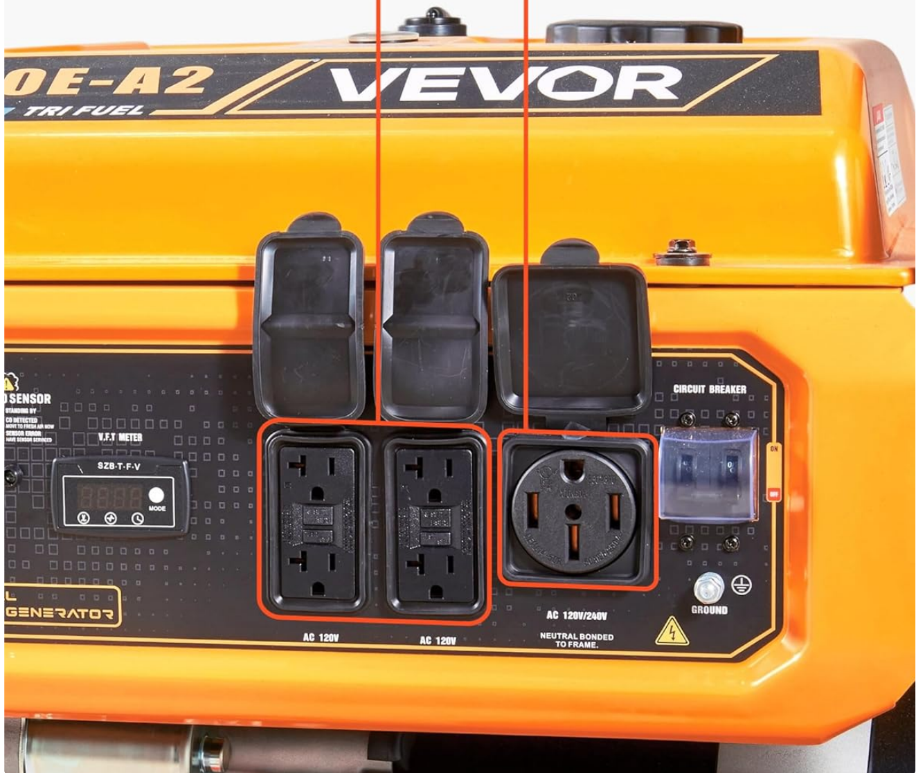
Figure 3: The control panel features multiple outlets, including 2x AC120V 20A household outlets and 1x AC120/240V 50A heavy-duty outlet.
