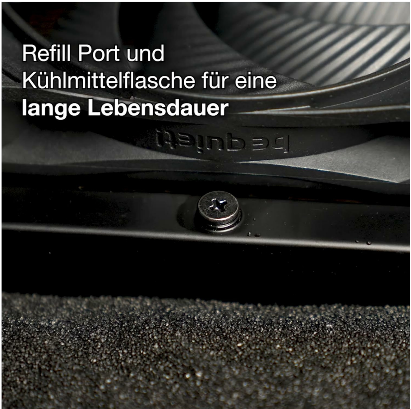
Image: Close-up of the refill port on the radiator, designed for easy coolant top-up.
